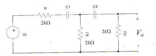
a) Ao can be calculated from the value of the transfer function when  $\omega \to \infty$   $H(j'\omega) = \frac{V_o(j'\omega)}{V_i'(j'\omega)} \xrightarrow{\omega \to \infty} A_o$ For  $\omega \to \infty$ , the circuit becomes:
