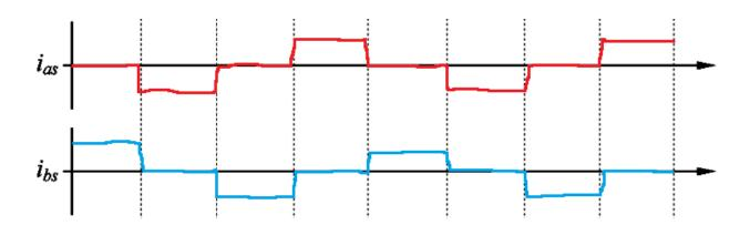
b) (40p) Sketch the sequence of currents  $i_{as}$  and  $i_{bs}$  to drive this motor at **half-step** in **CW** directions
