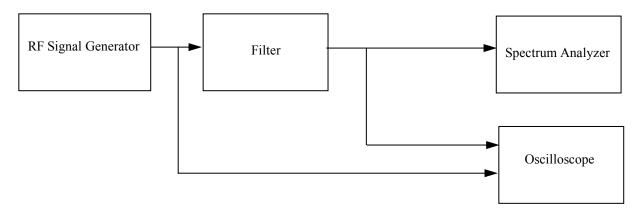
Figure 2: Experimental setup – Measurement of the frequency response of a filter.
