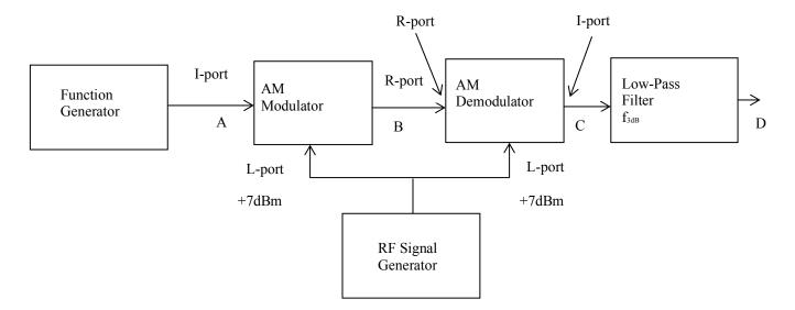
2. Devise and implement an op-amp-based low-pass filter that will eliminate the unwanted frequency component at the output of the second mixer. A Sallen-Key filter will likely provide the desired performance. You will need to determine the best value of the  $f_{MB}$  of the low pass filter (LPF) that will allow accurate recovery of an accurate replica of the modulating signal.
