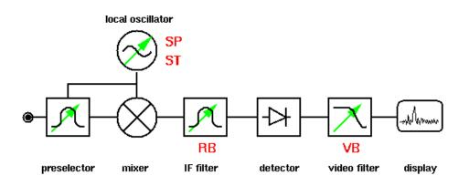
• The above figure shows the essential components required to illustrate the function and operation of a minimal swept-tuned spectrum analyzer.
