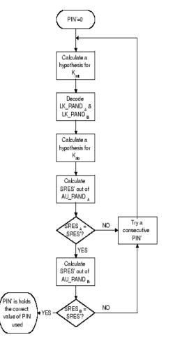
Figure 2: The PIN cracking algorithm [2].
