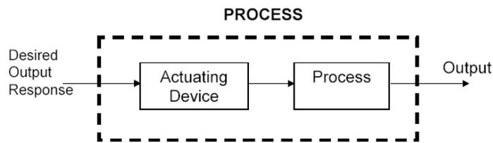
Figure 1.2 Open-loop Control System (without feedback)
