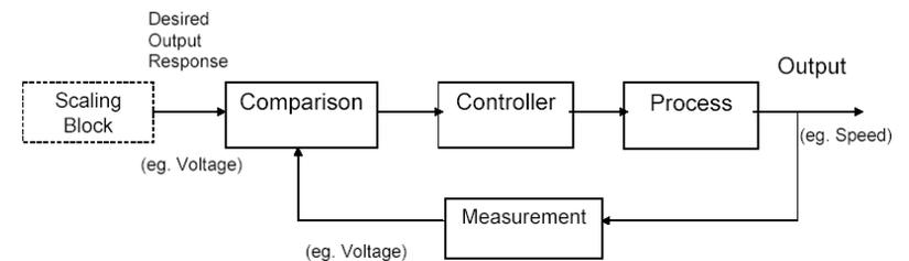
Figure 1.3 Closed-loop Control System (with feedback)
