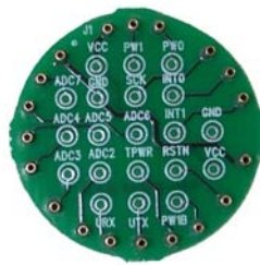
Figure 9-1. Photo of top-side of an MDA500CA for the MICA2DOT.
