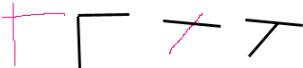
Figure 6: Example of drafting with Object Snap feature turned on.
