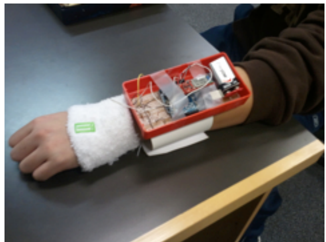
Figure 6. Low-Fi prototype, as worn during the experiment. The prototype weighs about 100g battery-included, the same as most cellphones, and this weight is distributed over a wide armband in order to increase comfort and not to create a new source of stress.
