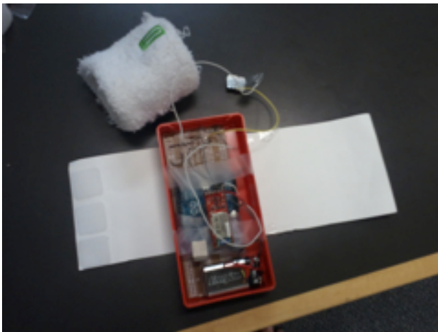
Figure 4. Form Factor, at rest. The prototype consists of a wide arm-band (for comfort and a secure grip) attached via velcro, the arduino board with the event recognition and broadcast logic embedded, a bluetooth modem, and the GSR sensor board and electrodes.
