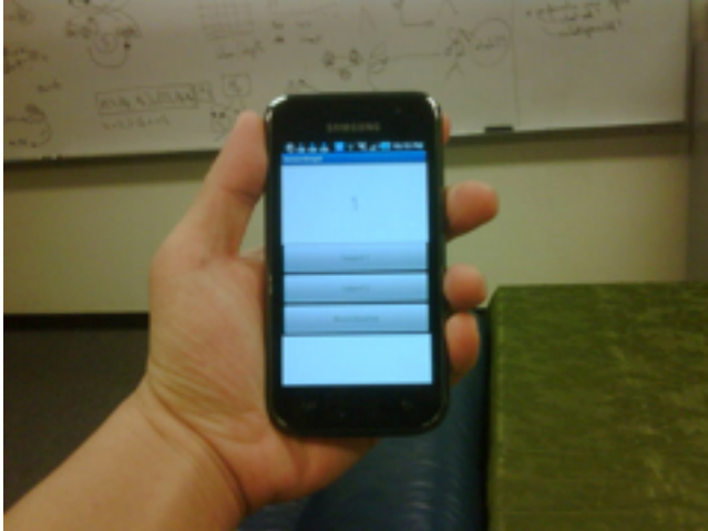
Figure 7. Android phone with experiment application (prisoner's dilemma game). Top Text Box: pay-off matrix and stress warning, Top Button: Defect, Middle Button: Cooperate, Bottom Button: Create Baseline.
