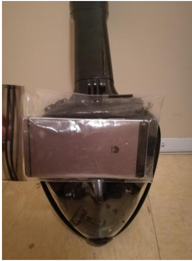
Figure 2: VR headset combines with sealed waterproof smartphone.
