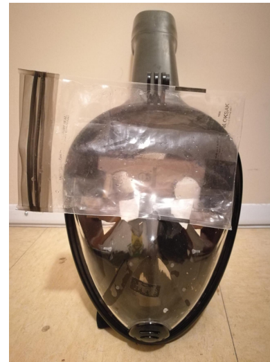
Figure 1: Basic structure of the underwater VR headset.
