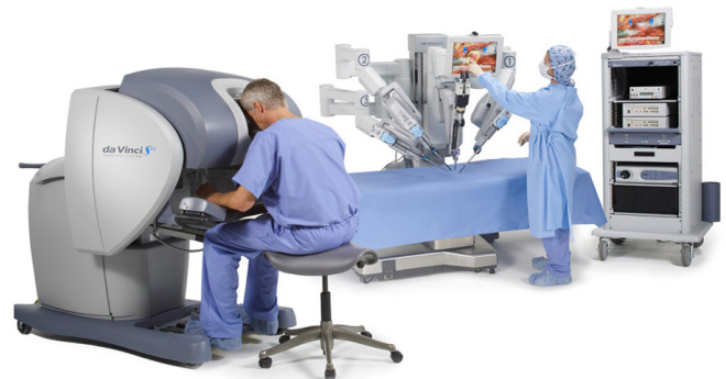
Figure 1: The surgeon at the console and the patient cart of the da Vinci Surgical System.
