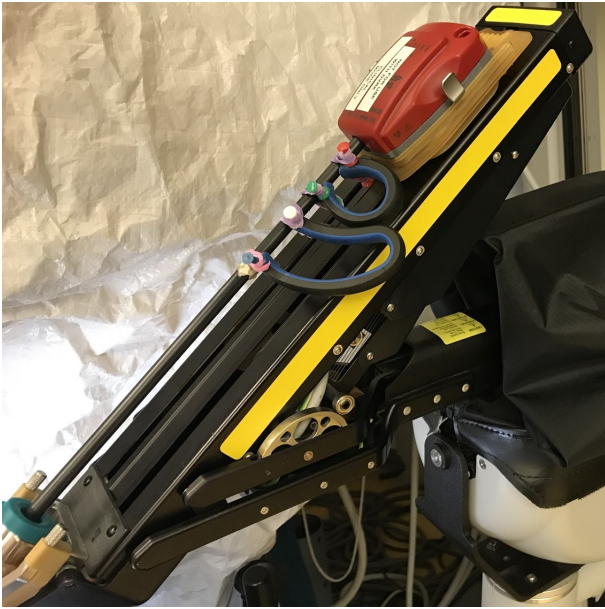
Figure 4: A closer view of one of the da Vinci PSMs after attaching a handle to make it easier for a user to hold.
