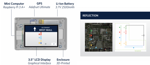
Figure 5: A Portable Device Prototype (Left) with a Navigation Interface and A Learning Reflection Interface (Right).
