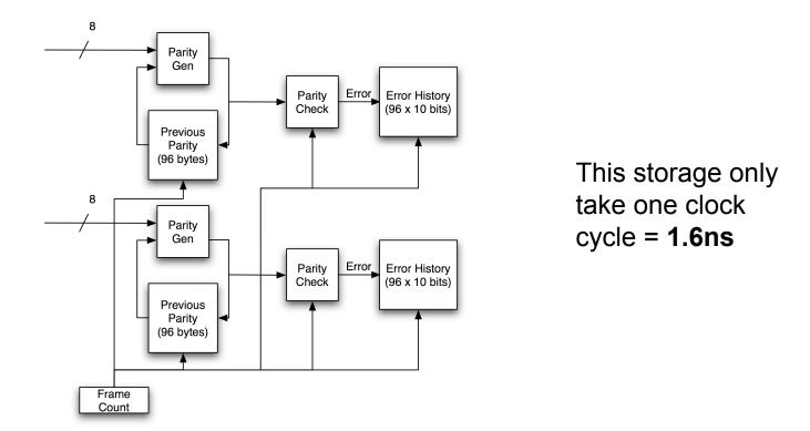
Using hardware we can easily evaluate the number of '1' in our 10-bit shift registers and determine if the threshold has been exceeded.
