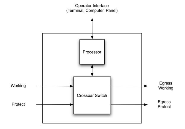
The basic design does not support automatic protection switching:
