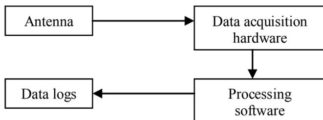
Fig. 1. Block diagram of the designed RF-detection RNG random oracle
