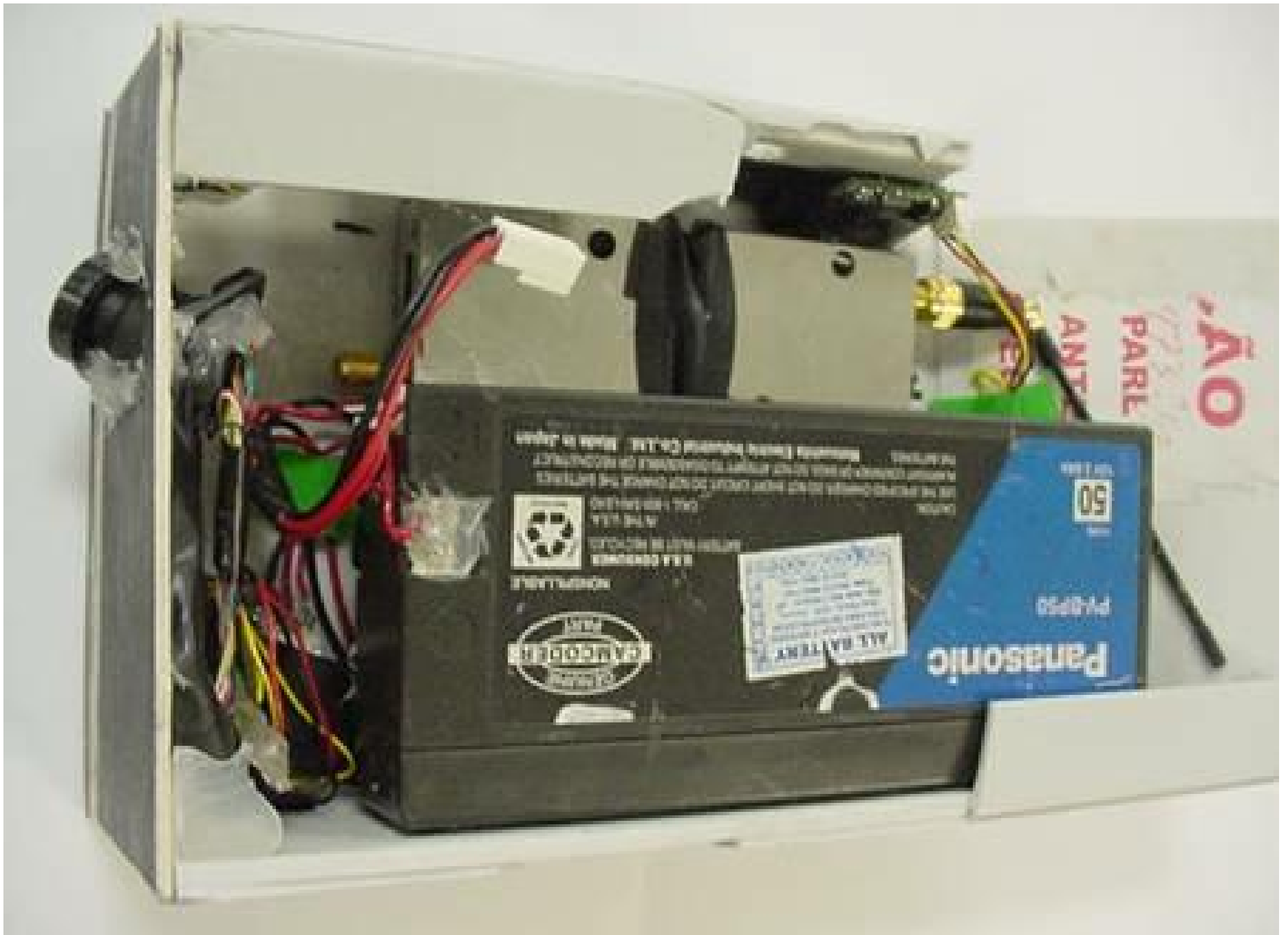
the camera has its own battery and transmission antenna
