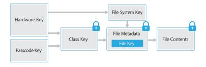
The content of a file is encrypted with a per-file key, which is wrapped with a class key and stored in a file's metadata, which is in turn encrypted with the file system key. The class key is protected with the hardware UID and, for some classes, the user's passcode. This hierarchy provides both flexibility and performance. For example, changing a file's class only requires rewrapping its per-file key, and a change of passcode just rewraps the class key.
