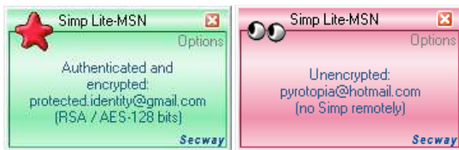
Figure 6. SimpLite-MSN provides usable security with recognizable dialog boxes displaying the security status of the instant messaging session. Green notifies the user of a secure session, while red notifies the user of an unsecure session.
