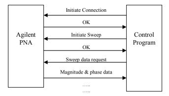
Fig. 2. Data acquisition protocol between PNA and controlling computer
