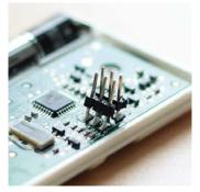
Fig. 1. Header pins soldered to ISP port
