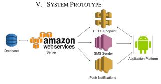
Fig. 3. High Level Design of the System Prototype
