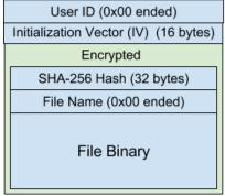
Fig. 2. File Wrapper and Encryption Format.
