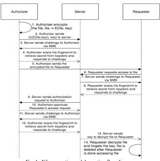
Fig. 1. File encryption and decryption flow diagram
