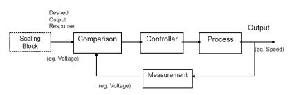
Figure 1.3 Closed-loop Control System (with feedback)
