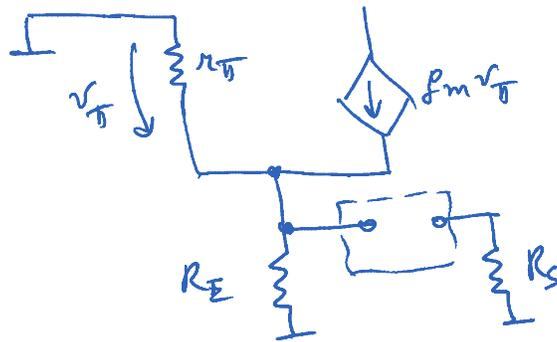
$$R_{E,ac} = \left( R_E \parallel \frac{r_{\pi}}{\beta+1} \right) + R_S = 52.2 \Omega + 50 \Omega = 102.2 \Omega$$
