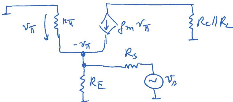
$$-v_{\pi} = \frac{R_E \parallel r_{\pi}}{R_s + R_E \parallel r_{\pi}} v_s + \beta_m v_{\pi} (r_{\pi} \parallel R_E \parallel R_s) \Leftrightarrow$$
