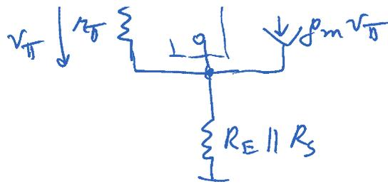
$$R_{\pi, oc} = R_E \parallel R_S \parallel \frac{r_{\pi}}{\beta + 1} \approx 50\Omega \parallel 53\Omega \approx 25.2\Omega$$
