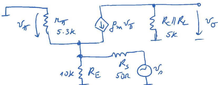
$$-v_{\pi} = \frac{R_E \parallel \frac{r_{\pi}}{\beta+1}}{R_s + R_E \parallel \frac{r_{\pi}}{\beta+1}} v_s$$
