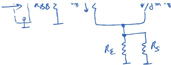
$$R_{B,ac} = R_{BB} \parallel (r_{\pi} + (\beta+1) R_E \parallel R_S)$$
