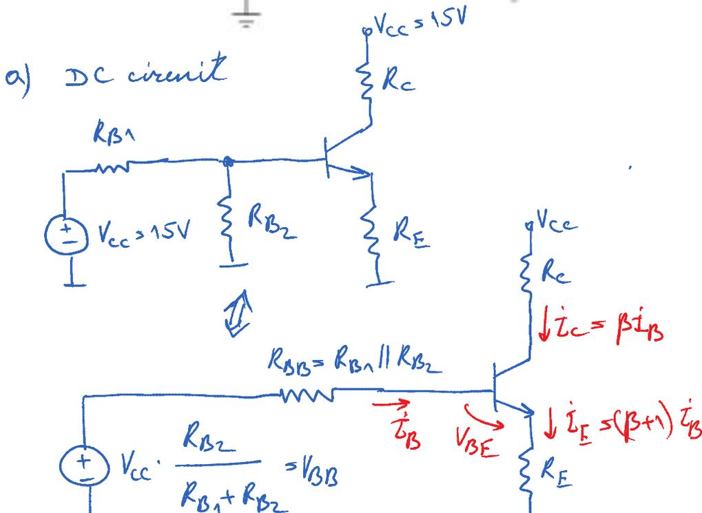
$$V_{CC} \cdot \frac{R_{B2}}{R_{B1} + R_{B2}} = V_{BB}$$
