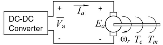
b) (10pts): Assume the same PM dc machine as in a). Sketch a DC-DC converter circuit and clearly label all its components assuming that that can drive this motor:
