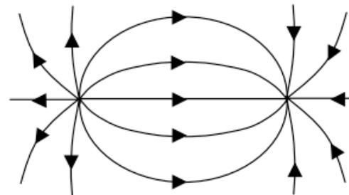
Electric dipole with positive charge on left
