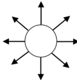
Positively charged conducting sphere
