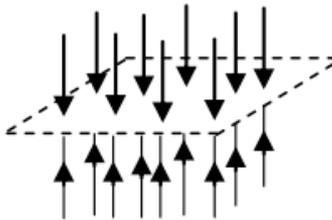
Infinite plane of negative charge
