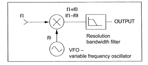
As the  $f_0$  increases, the spectrum of the input signal is translated past the centre frequency of the resolution bandwidth filter. For practical reasons, we normally must employ a bandpass filter rather than the low pass filter shown.
