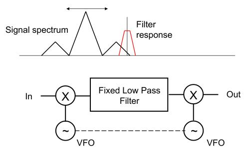
Although one appears to be shifting the corner frequency of the filter, one is actually translating the spectrum of the signal!
