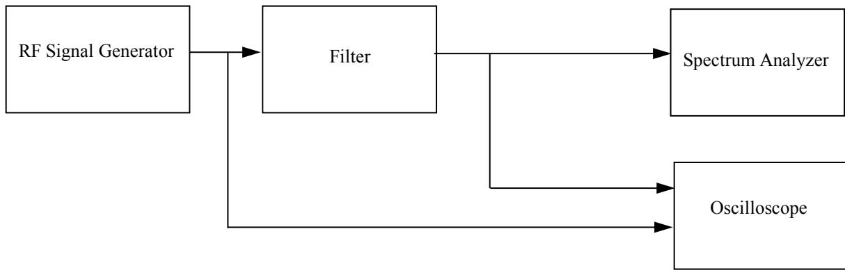
Figure 2: Experimental setup – Measurement of the frequency response of a filter.
