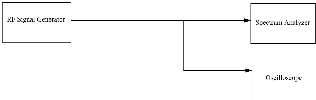
Figure 1: Experimental setup – measurement of the power spectrum.
