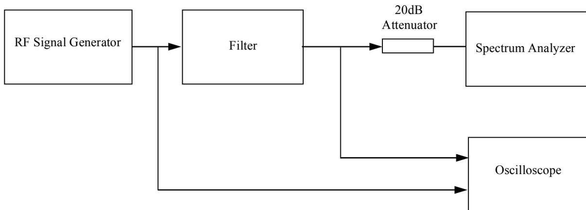
Figure 2: Experimental setup – Measurement of the frequency response of a filter.
