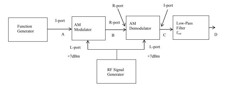
2. Devise and implement an op-amp-based low-pass filter that will eliminate the unwanted frequency component at the output of the second mixer. A Sallen-Key filter will likely provide the desired performance. You will need to determine the best value of the  $f_{3dB}$  of the low pass filter (LPF) that will allow accurate recovery of an accurate replica of the modulating signal.
