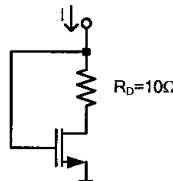
Sat. condition :  $V_{GD} \leq V_{th}$
