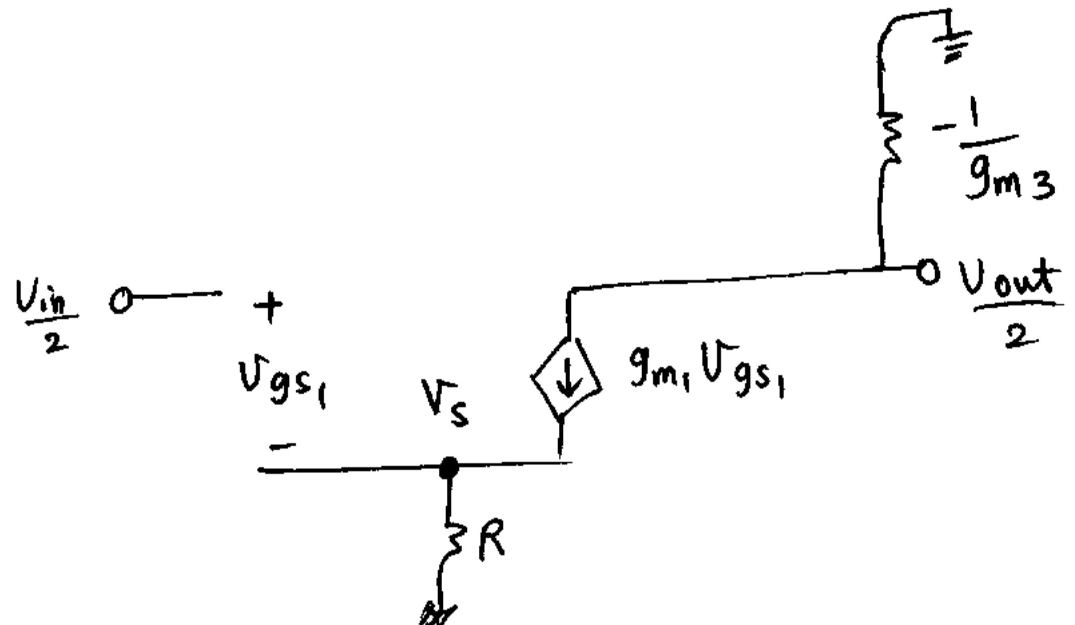
$$\frac{V_{out}}{2} = \left( -\frac{1}{g_m 3} \right) (-g_m 1, V_{gs1}) = \frac{g_m 1}{g_m 3} V_{gs1}, \quad (I)$$
