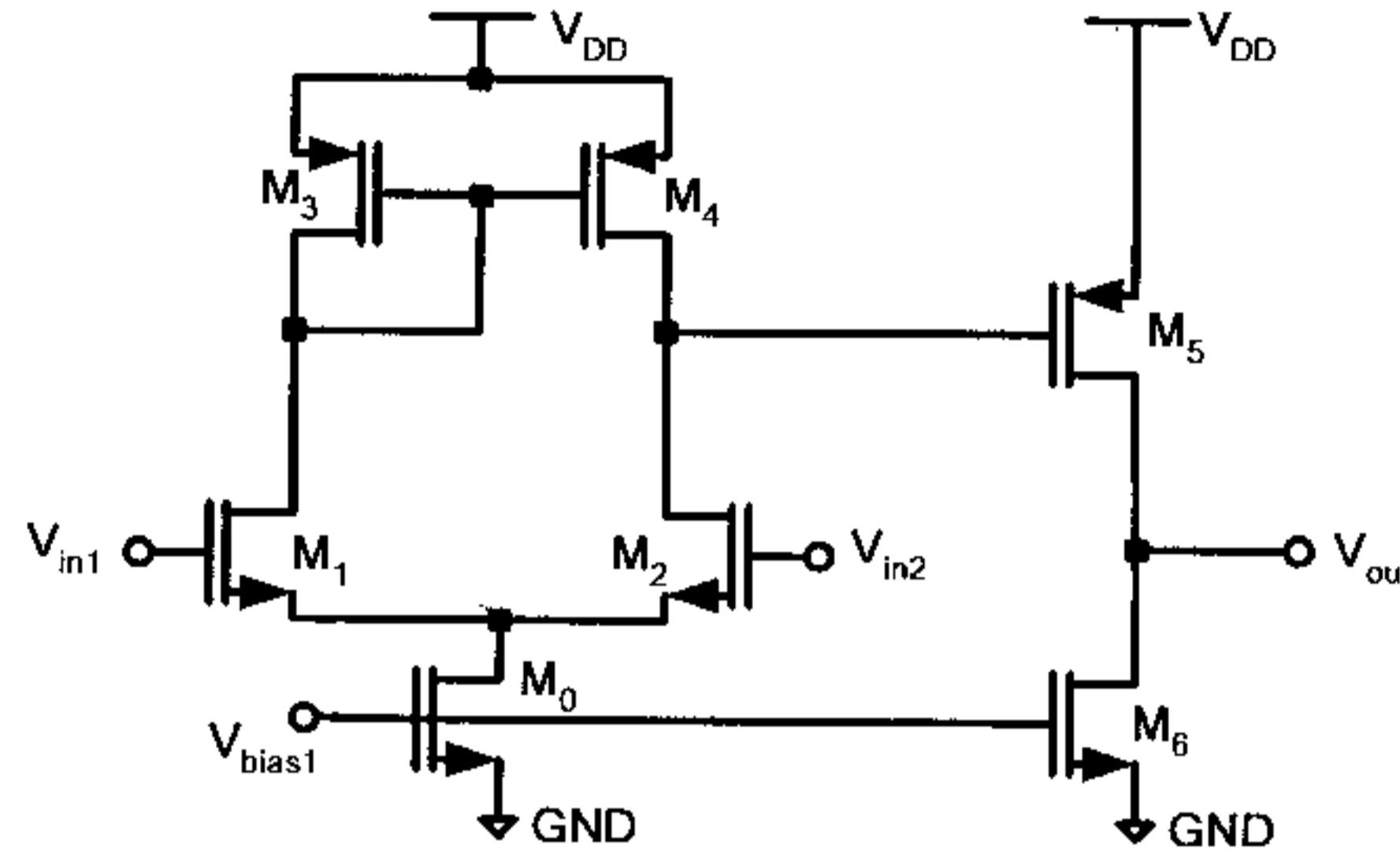
$$I_6 = 0.5 \text{ mA} = \frac{1}{2} \times 1 \times \frac{W_6}{0.4} \times V_{OD6}^2 = \frac{1}{2} \frac{W_6}{0.4} (0.2)^2 \rightarrow W_6 = 10 \mu\text{m}$$
