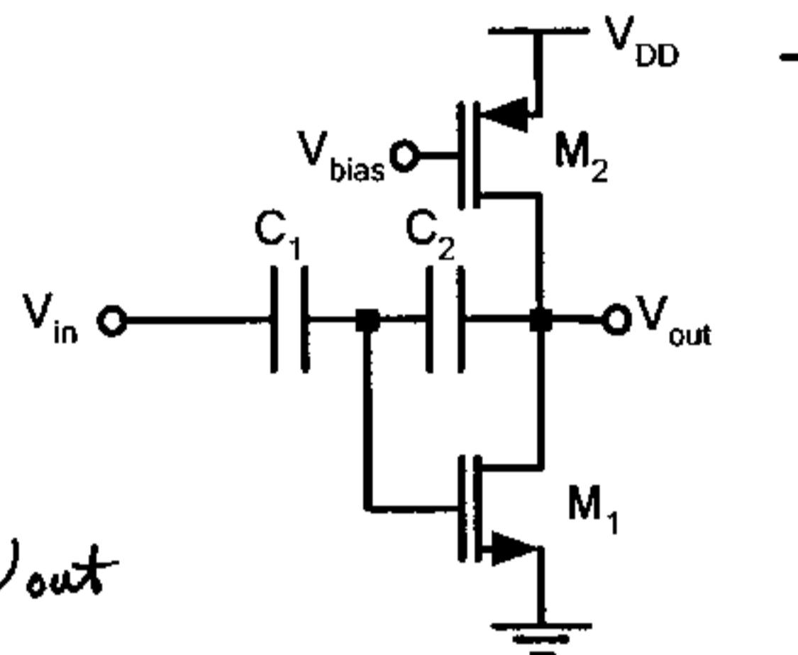
$$I_x = g_m1 V_{gs1} \rightarrow V_{gs1} = \frac{I_x}{g_m1}$$
