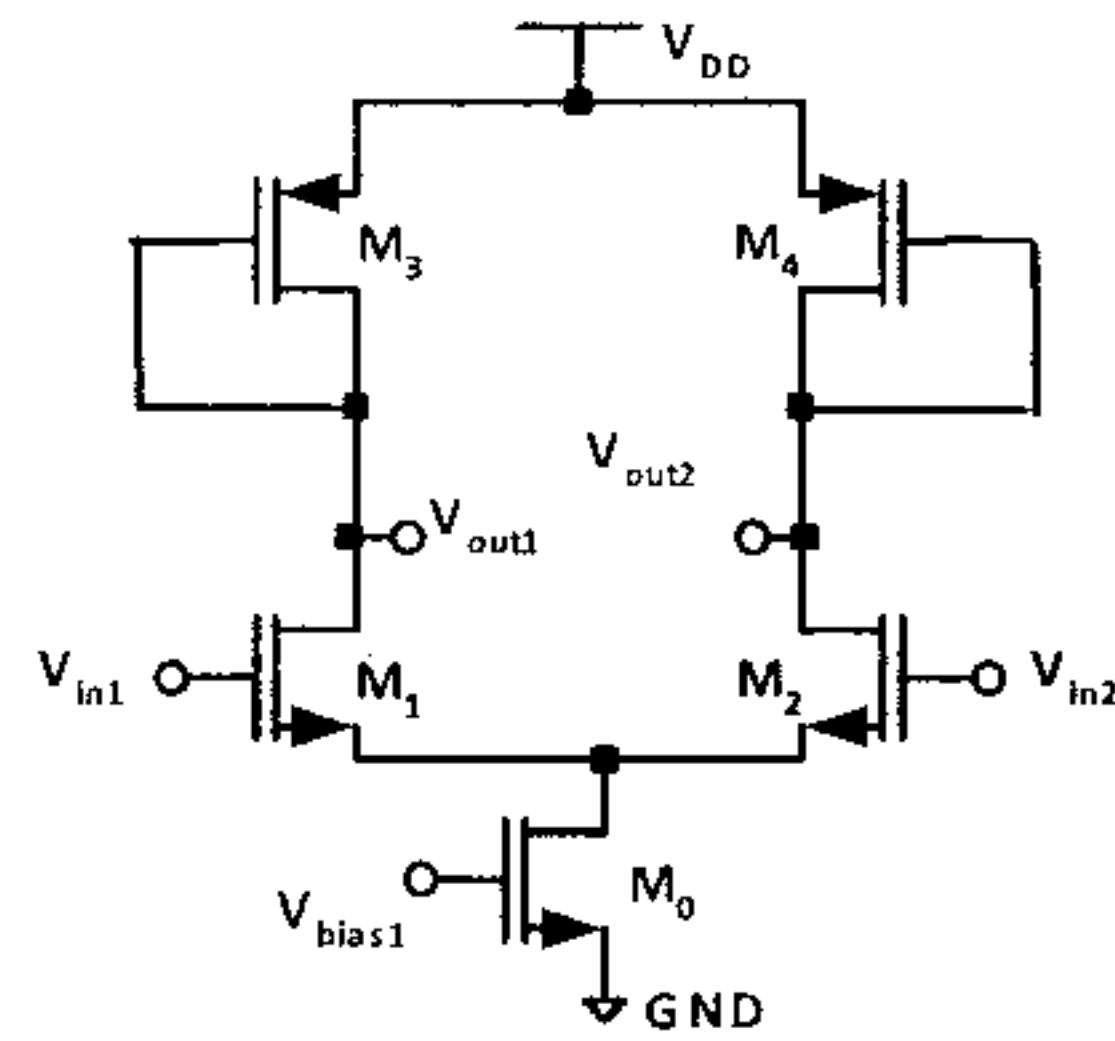
$$I_{D1} = 0.5 \text{ mA} = \frac{1}{2} \times 1 \times \frac{640}{0.4} (V_{GS1} - 0.5)^2 \rightarrow V_{GS1} = 0.525 \text{ V}$$
