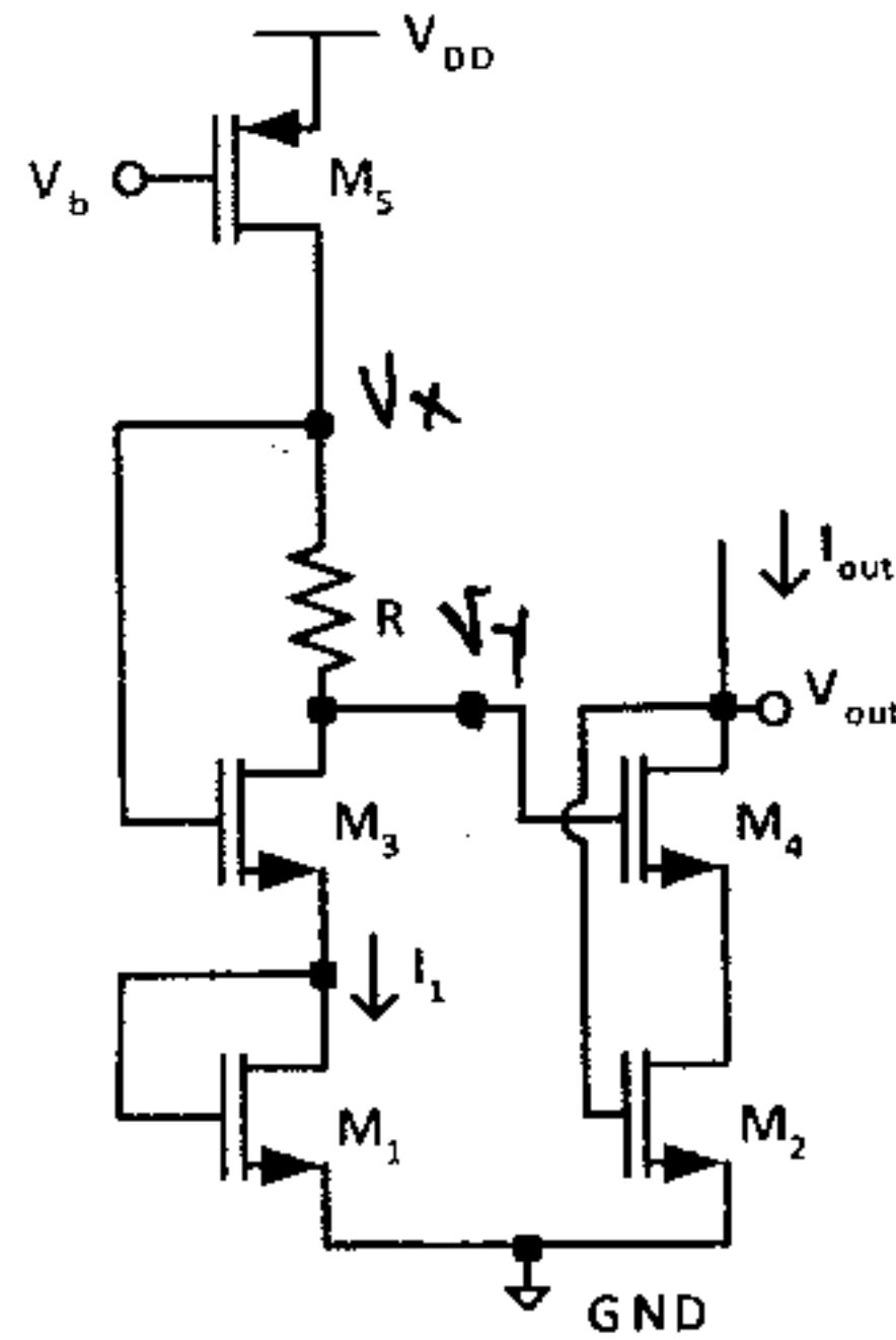
$$I_{out} = I_5 = \frac{1}{2} \mu_p C_{ox} \left( \frac{W}{L} \right) (V_{GS5} - |V_{th}|)^2 = \frac{1}{2} \times 0.25 \times 40 (3 - 2.3 - 0.5)^2 = 0.2 \text{ mA}$$
