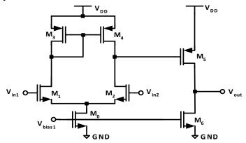
Find V<sub>bias1</sub>, and all the transistor widths (i.e., W<sub>0</sub>, W<sub>1</sub>, W<sub>2</sub>, W<sub>3</sub>, W<sub>4</sub>, W<sub>5</sub>, W<sub>6</sub>).
