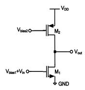
Assuming both transistors are in saturation, find the following values:
