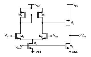
For your convenience the circuit diagram and transistor parameters are replicated here:  $\lambda_{(NMOS)} = \lambda_{(PMOS)} = 0.1 \text{ V}^{-1}, \gamma = 0, V_{DD} = 3 \text{ V}, V_{TH(NMOS)} = |V_{TH(PMOS)}| = 0.5 \text{ V}, \mu_n C_{ox} = 1 \text{ mA/V}^2, \mu_p C_{ox} = 0.5 \text{ mA/V}^2.$
