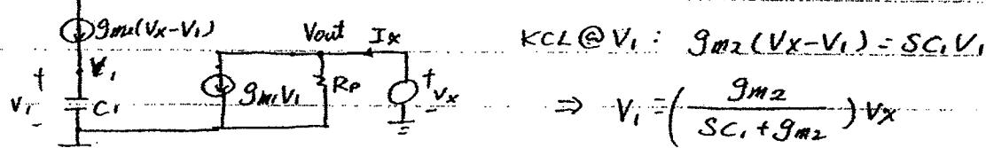
$$\text{KCL at } V_1: g_{m2}(V_x - V_1) = g_{m1}V_1$$
