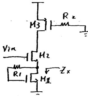
$$\frac{V_{out}}{V_{in}} = \frac{g_{m2} (r_{o3}/(1+g_{m2}r_{o2})Z_x)}{1 + g_{m2}Z_x} \approx \frac{g_{m2}(r_{o3}/r_{o2})}{1 + \frac{g_{m2}}{g_{m1}}} \rightarrow \infty \text{ if } \lambda = 0$$
