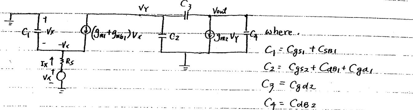
$$\text{KCL @ } V_{\text{out}} : SC_3(V_Y - V_{\text{out}}) = g_{m2}V_Y + SC_4V_{\text{out}}$$
