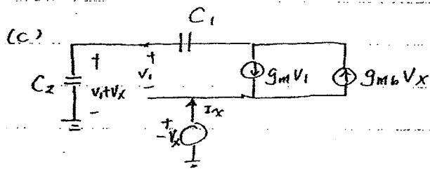
$$S C_2 (V_i + V_x) + g_m V_i = g_{mb} V_x$$
