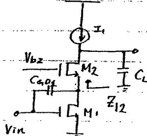
The impedance  $Z_{12}$  can be derived from the following small signal model
