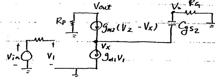
$$\text{KCL at } V_2 : \frac{V_2}{R_g} = sG_{gs2}(V_x - V_2)$$
