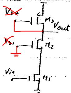
The impedance @  $V_{out}$  =  $\frac{1}{g_{m_3}}$
