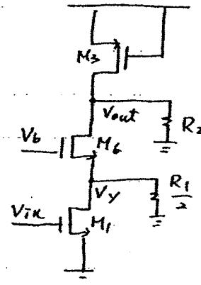
$$\frac{V_y}{V_{in}} = -g_{m1} \left( \frac{1}{g_{m6}} // \frac{R_1}{2} \right), \quad \frac{V_{out}}{V_y} \approx +g_{m6} \cdot R_2$$
