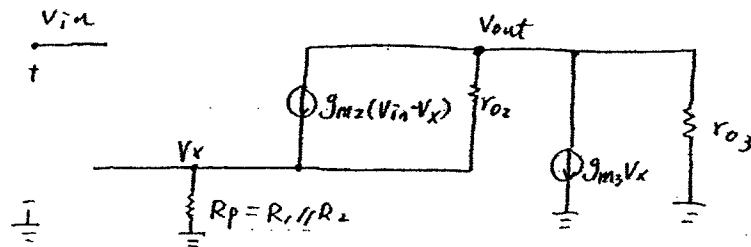
$$\text{KCL at } V_x, V_{out} : \frac{V_x}{R_p} = g_{m2}(V_{in} - V_x) + \frac{V_{out} - V_x}{r_{o2}} = -(g_{m3}V_x + \frac{V_{out}}{r_{o3}})$$
