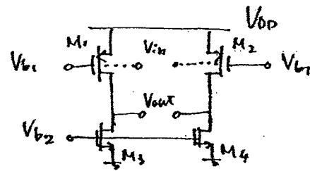
(c)  $g_{mb} = g_m \frac{\gamma}{2\sqrt{|\beta\phi_F| + |V_{SB}|}}$
