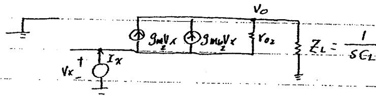
$$\text{KCL @ } V_o : \frac{V_o}{Z_L} + \frac{V_o - V_x}{r_{o2}} = (g_{m2} + g_{mb2})V_x \Rightarrow \left( \frac{1}{Z_L} + \frac{1}{r_{o2}} \right) V_o = (g_{m2} + g_{mb2} + \frac{1}{r_{o2}}) V_x$$
