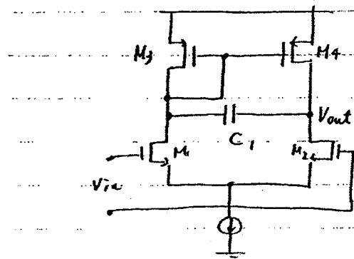
C<sub>1</sub> is like an open circuit @ very low frequency
