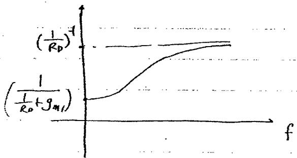
$$\text{KCL at } V_{out}: I_x = \frac{V_x}{R_o} + g_{m1}V_1$$
