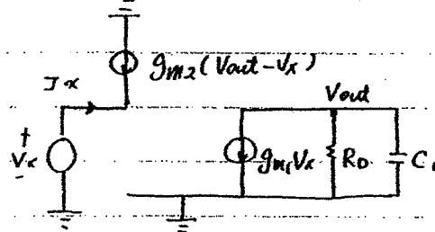
$$V_{out} = -g_{m1}V_x \left( R_o \parallel \frac{1}{g_{m1}} \right)$$
