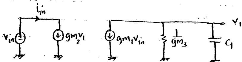
$$Z_{in} = \frac{V_{in}}{I_{in}} = \frac{V_{in}}{g_{m2}V_1} \quad V_1 = -g_{m1} \left( \frac{1}{C_s + g_{m3}} \right) V_{in}$$
