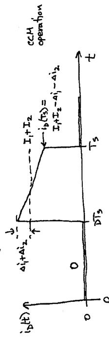
$$\text{peak } i_d(t) = I_1 + I_2 + \Delta i_1 + \Delta i_2$$
