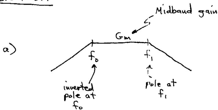
$$G(s) = \frac{G_m}{\left(1 + \frac{s}{\omega_1}\right)\left(1 + \frac{\omega_0}{s}\right)} \quad \text{with } \omega_0 = 2\pi f_0$$
