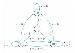
3. Design the binary multiplier controller shown below using multiplexors, a decoder, and a register.
