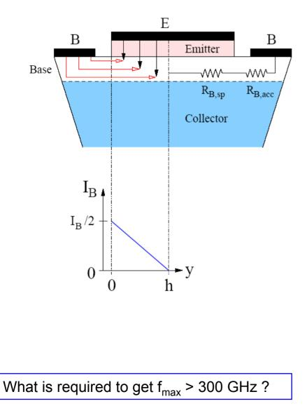
$$\begin{aligned} P_{\text{left}}(y) &= I_B(y)^2 R\\ P_{\text{left}} &= \int_0^h \frac{I_B^2}{4} \left(1 - \frac{y}{h}\right)^2 \frac{\rho \, dy}{A} \end{aligned}$$
