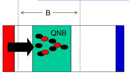
$$Q_{E,b}(V_{BE}) = -q \frac{1}{2} W_B A \left[ n_{0p} \exp(\frac{V_{BE}}{V_{th}}) - n(W_B) \right] - q W_B A n(W_B)$$
