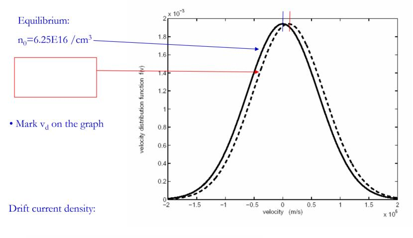
$$\begin{aligned} \vec{J}_{e,\text{drift}} &= \vec{J}_{e,\text{drift}\rightarrow} + \vec{J}_{e,\text{drift}\leftarrow} \\ &= -q\frac{n}{2}\left(2\vec{v}_R + \vec{v}_{de}\right) + \left(-q\frac{n}{2}\left(-2\vec{v}_R + \vec{v}_{de}\right)\right) \\ &= \end{aligned}$$
