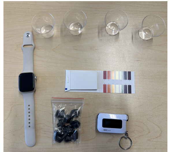
Figure 1: Illustration of the components of the detection system, which includes pH test paper, a pH indicator, a breathalyzer, mouth pieces for the breathalyzer. The experiment setup also uses an Apple watch for heart rate measurement, and plastic cups to hold saliva samples.
