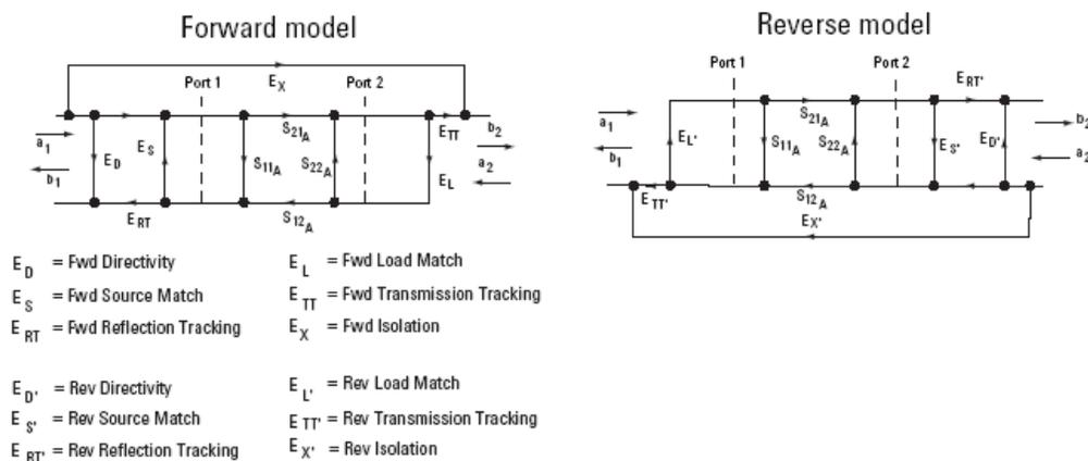
$$S_{11a} = \frac{\left(\frac{S_{11m} - E_D}{E_{RT}}\right)\left(1 + \frac{S_{22m} - E_{D'}}{E_{RT'}} E_S'\right) - E_L \left(\frac{S_{21m} - E_X}{E_{TT}}\right)\left(\frac{S_{12m} - E_{X'}}{E_{TT'}}\right)}{\left(1 + \frac{S_{11m} - E_D}{E_{RT}} E_S\right)\left(1 + \frac{S_{22m} - E_{D'}}{E_{RT'}} E_S'\right) - E_L' E_L \left(\frac{S_{21m} - E_X}{E_{TT}}\right)\left(\frac{S_{12m} - E_{X'}}{E_{TT'}}\right)}$$
